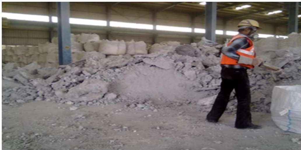
Figure 1. Manual collection of aluminium dross.
