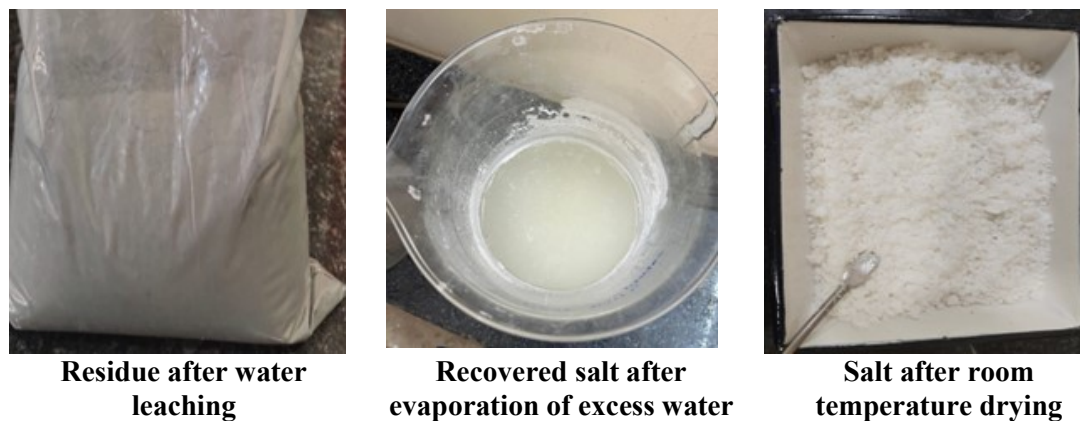
Figure 6. Residue and salt after leaching.
